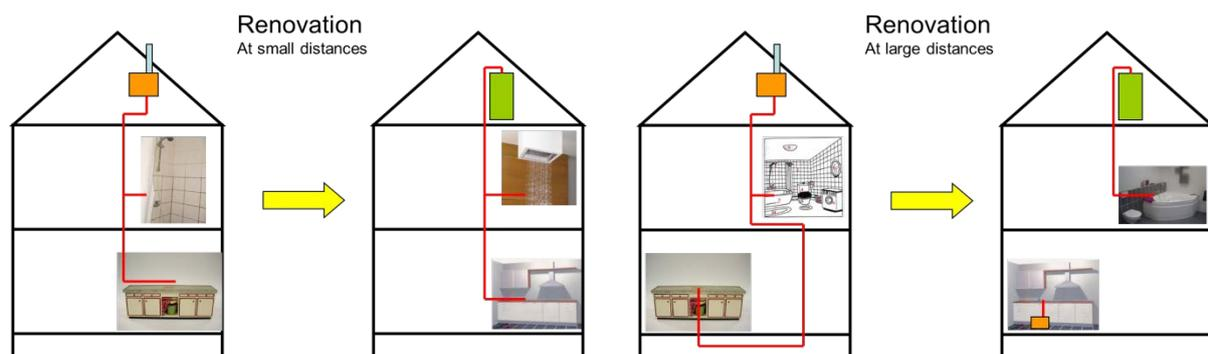
**Figure 10: Renovation option in situation of small and large distances (=> separate appliances) between bathroom and kitchen**
