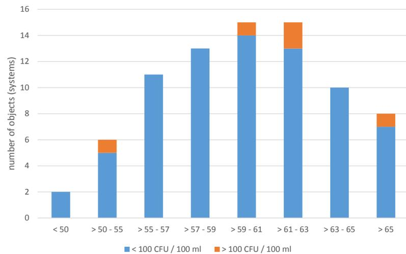
Number of objects, divided according to temperature at the outlet of the water heater (storage) and number of samples > 100 CFU / 100 ml. based on data from Rühling et al. 2018 (p. 40-41).
