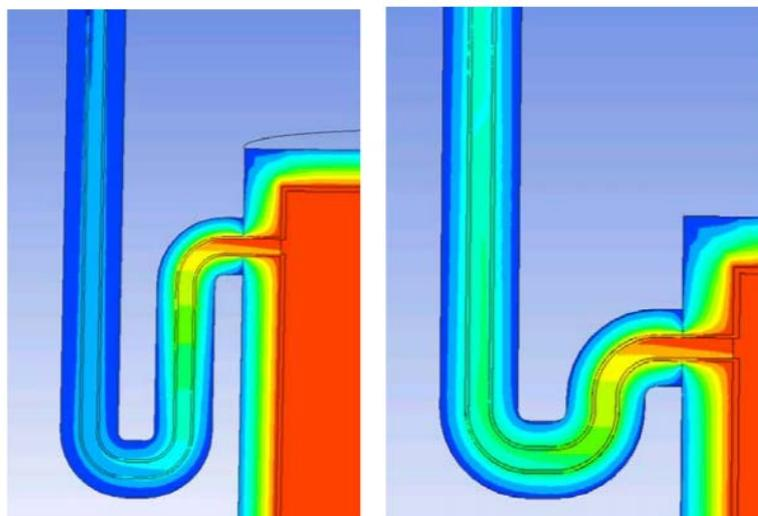
*Effective (left) and only partially effective (right) heat trap of a storage tank pipe connection. According to Haller & Battaglia (2017).*
