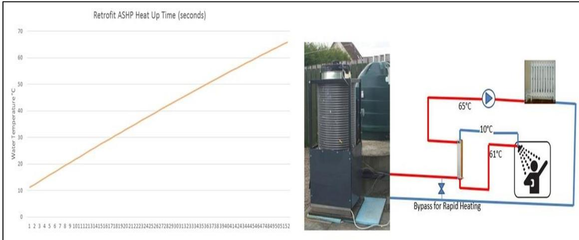
Figure 10 Time required to overcome thermal mass: Retrofit conditions
