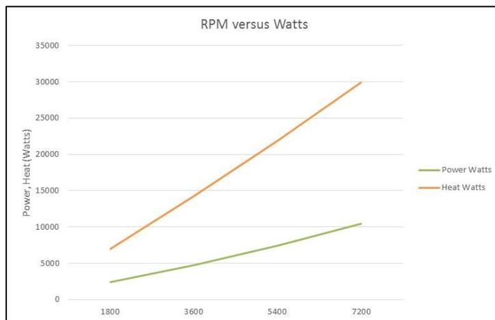
Figure 6 Typical performance of domestic compressor : RPM vs Power and RPM vs Heat
