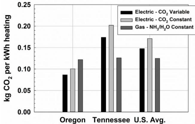
Fig. 6. Comparison of CO<sub>2</sub> Emissions of Gas-fired and Electric HPWHs Ambient of 20°C and a Temperature Lift of 45 K.
