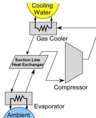
Fig. 2. Schematic of CO<sub>2</sub> Vapor Compression Heat Pump Water Heater
