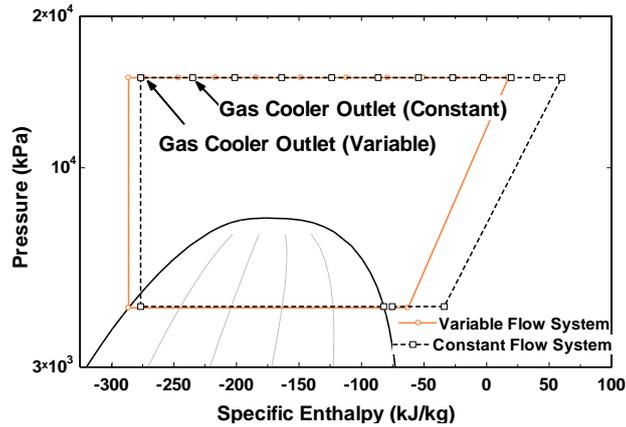
Fig. 3. Pressure-enthalpy Diagram of Baseline CO<sub>2</sub> Heat Pump Cycles
