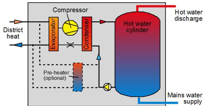
Figure 1.2 Basic layout of a booster heat pump.
