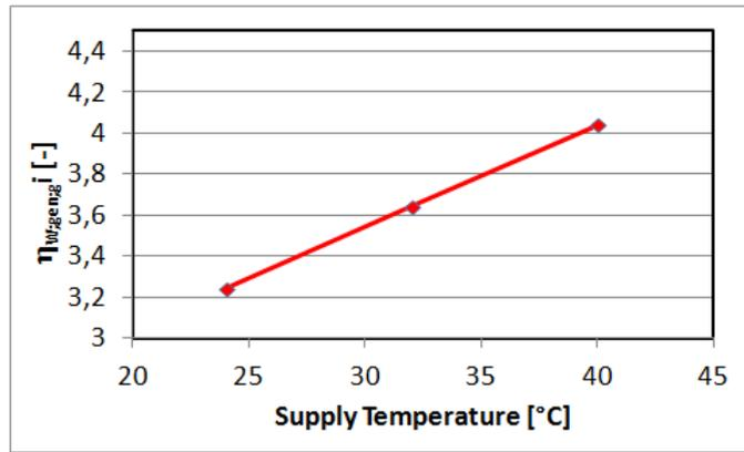
Figure 1.3  $\eta_{w,gen,gi}$  of a booster heat pump, as tested by KIWA for a tap water heat demand of 14 GJ(class 4, according to NEN 7120).
