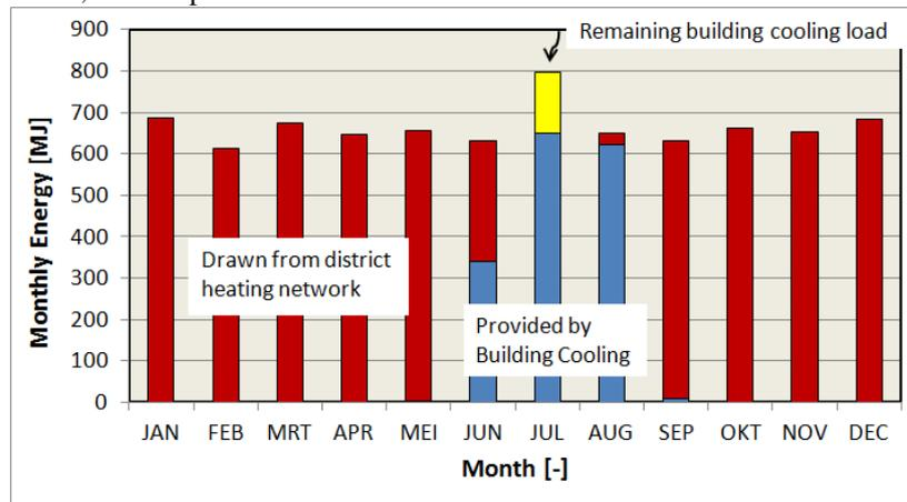
Figure 5.2 Graphical representation of energy need from the district heating network (red), thermal energy provided by building cooling (blue) and remaining cooling demand (not utilised as heat source for the booster heat pump, yellow). In this case ( $A_g=150$ m<sup>2</sup>), the equivalent COP for summer cooling = 3660.
