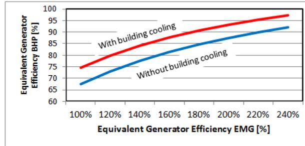
Figure 5.1 Booster heat pump efficiency, with and without building cooling, depending on district heating generation efficiency, for  $A_g=150$  m<sup>2</sup>, COP=4,04 @ 14000 MJ.
