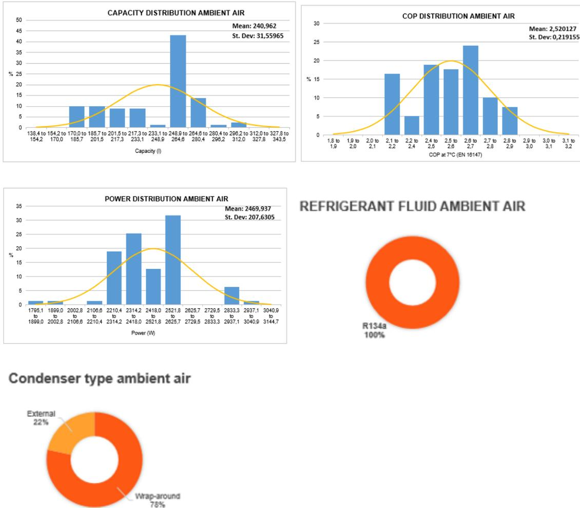
Fig 2.1 Characteristics of ambient air HPWH's
