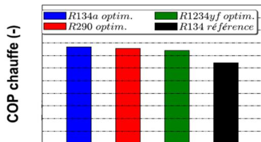
In a second step, the HPWH components were optimized for each type of refrigerant (compressor size, condenser and evaporator heat transfer surfaces). Results are shown on the figure 3.2. One can see that if the machines are redesigned, the alternative refrigerants are really suitable for DHW production. This study also shows that the alternative refrigerants lead to a reduced load for the same performance.
