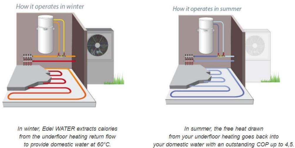
Fig 2.3 Function of HPWH on underfloor system
