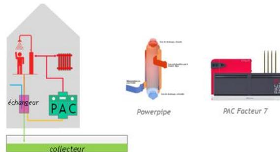
Another study realised by CSTB [8] describes two types of configuration to recover energy from grey water at building scale : one configuration without any storage, with a system like a Powerpipe®, and one configuration with storage (PAC F7®).
