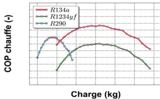
A first step was to study the COP for a water heating phase from 10°C to 55°C of an air-source HPWH equipped with R134a and then, in drop-in operation, with R1234yf and R290. Figure 3.1 shows the COP depending on the refrigerant charge for this R134a reference HPWH. Obviously, the COP is higher for R134a as the HPWH was designed for this refrigerant. However, the performances degradation is relatively low, taking in account this purely drop-in operation.
