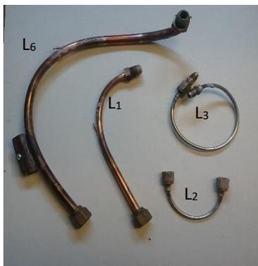
Figure 2. Connection lines. L<sub>6</sub> and L<sub>1</sub> with immersed temperature pockets. L<sub>2</sub> and L<sub>3</sub> ss-tubes without. L<sub>6</sub> with fitting for expansion valve bulb.
