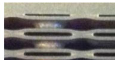
Figure 6. Cut section of test plates where solder wetting was examined.
